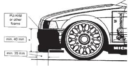
1:1 car construction to absorb impact energy.
